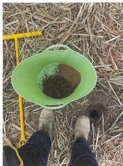
Identifying varying soil types during soil sampling
