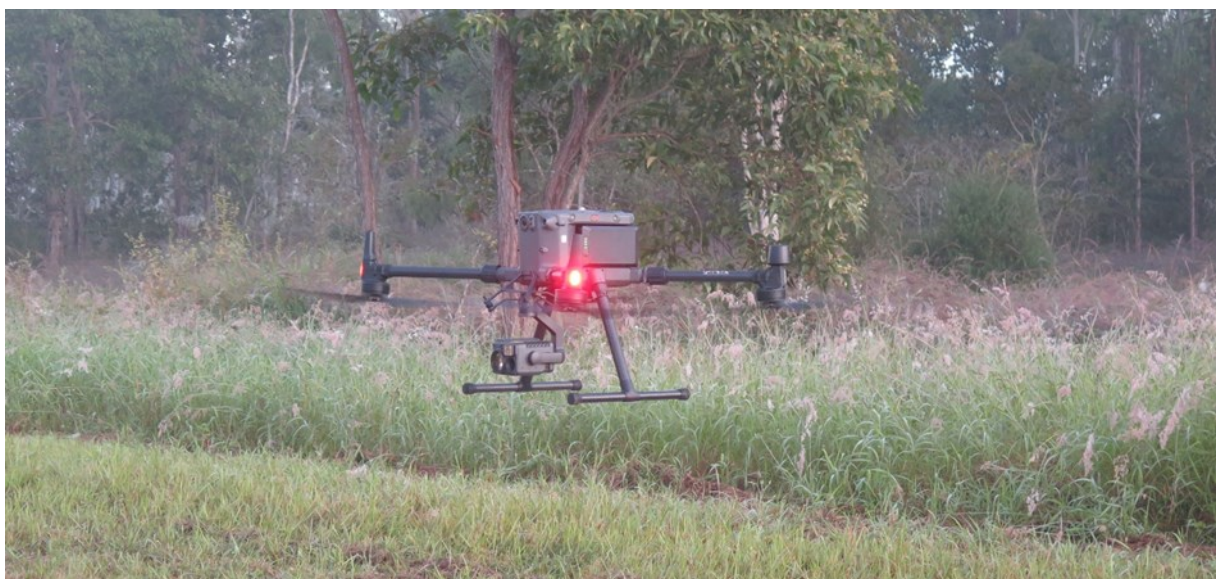
Photo 3 (above): DJI Matrice 300 RTK drone with H20T camera system used in the trial.
