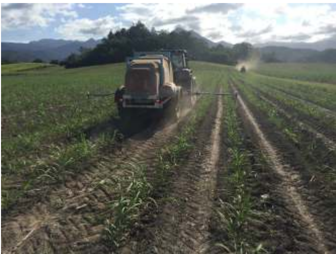
Above: Broadcast application using a boom spray
