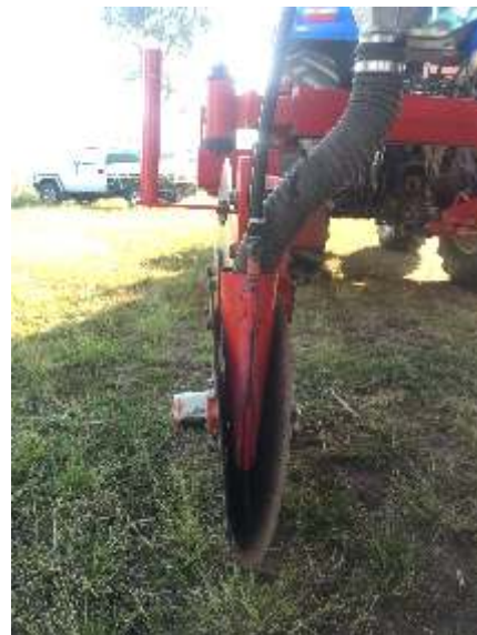
Left: In-furrow injection using a stool splitter when fertiliser is applied.
