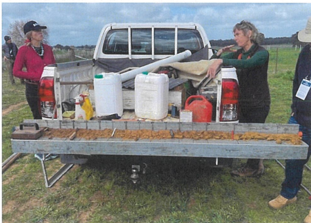
Deep core soil sampling Left is top soil – right is sub soil
