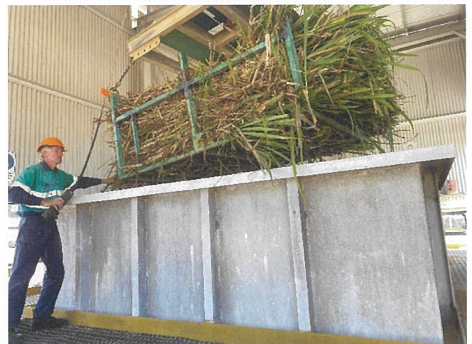
Below: Whole stalk material being lowered into a HWT tank
