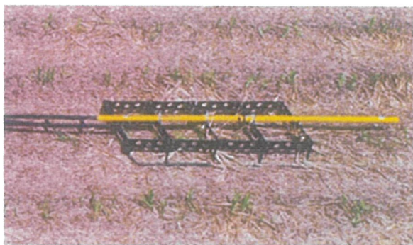
New Sled and DualEM 421S collecting EC data.
