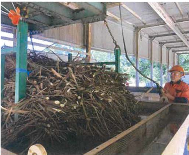
William Tiento at the Hot Water Treatment Tanks
