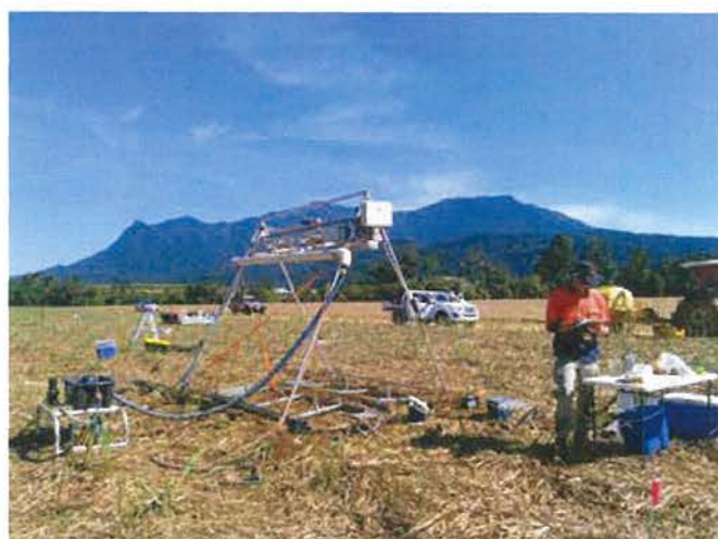
Rainfall Sim used to simulate heavy rainfall to capture information on how certain chemicals behave under typically wet conditions
